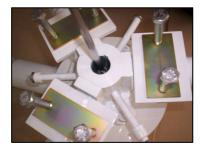
Using a hexagon key, fit the front shaft bolt (15) and washer (14) to the spring locking washer provided into the generator shaft and tighten the assembly.
