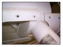
Slide the nacelle cover (0730) along the boom so that it is covering the generator. Secure the nacelle cover to the rear of the generator with the two M6 screws to the required torque setting (see 3.4 Pg 7). Slide the front closing plate between the underside of the generator and the nacelle cover and secure with the four M5 screws to the required torque setting (see 3.4 Pg 7) through the holes provided.
