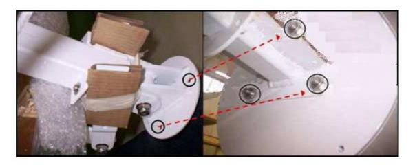
Now fit the four lower bolts (20), washers (19) and nuts (18) on to the generator sides by means of the side bars. Level the boom with the generator, secure the bolts through the rubber bushes so that the boom is held in place and tighten all fastenings to the required torque setting (see 3.4 Pg 7).
