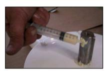
Smear waterproof grease (30) over the shaft and insert a little inside the front of the generator where the shaft projects out.
