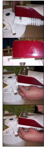
g) Now fit the nose cone (10) over the three spokes and fit the three Nylock nuts (16) and washers (17).
