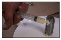
Smear waterproof grease over the shaft
