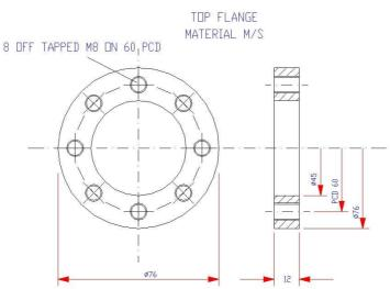
Four bolts are supplied for mounting of the e220 unit, however eight holes have been provided to allow interchange-ability between all Kestrel units. Secure the assembled e220 unit by using holes 1, 3, 5 and 7 as shown along side, and the M8 Hi-Tensile bolts with spring washers.
