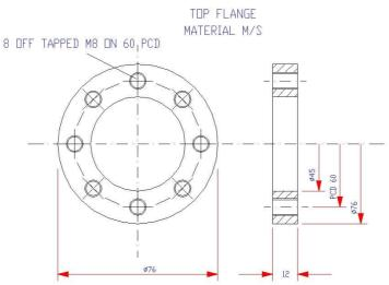
Four bolts are supplied for mounting of the e150 unit, however eight holes have been provided to allow interchange-ability between all Kestrel units. Secure the assembled e150 unit by using holes 1, 3, 5 and 7 as shown along side, and the M8 Hi-Tensile bolts with spring washers.
