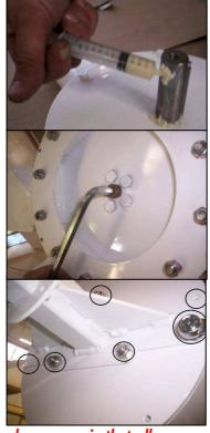
Do not over-tighten such that the tail boom is crushed or distorted. Check once again that all bolts are fitted and tightened to torque settings (section 3.3).
